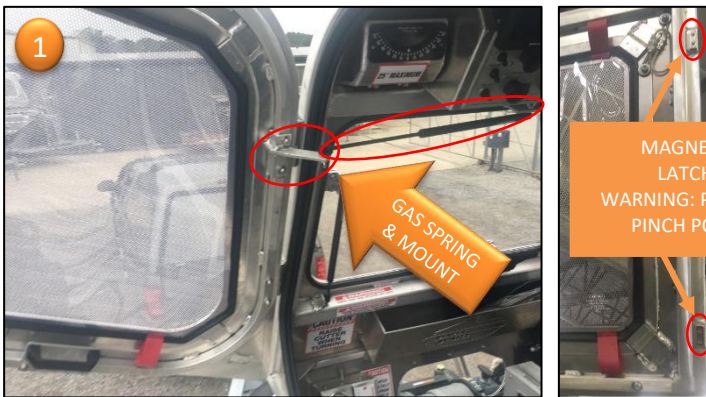
GAS SPRING, MOUNT, AND MAGNETIC LATCH DESIGNED SUCH THAT DOOR EASILY OPENS WITH A BUMP OF THE HAND.
