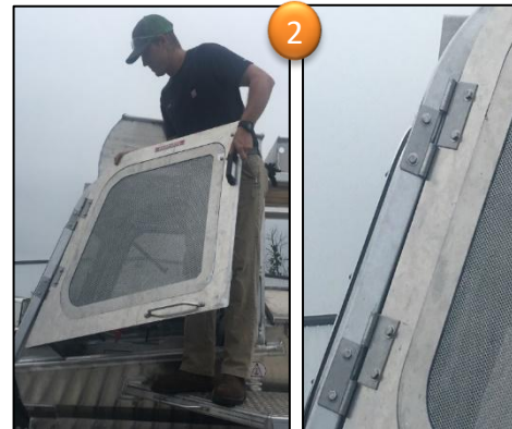
DOOR MOUNTS TO MARSH MASTER® ON "LIFT-OFF" HINGES. SEE CAB DOOR REMOVAL PROCEDURE SECTION FOR DOOR REMOVAL PROCEDURE
