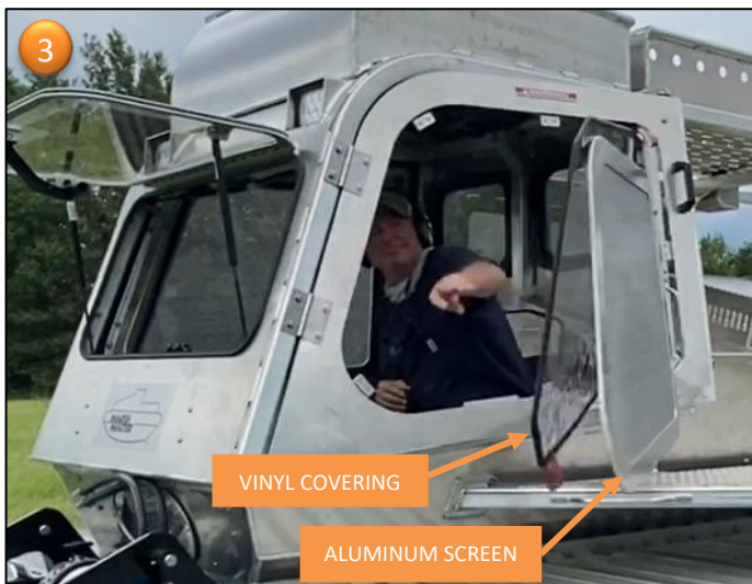
VINYL COVERING AND ALUMINUM SCREEN DESIGNED SUCH THAT A STRONG PUNCH WILL DISLodge FROM DOOR FRAME ALLOWING FOR CAB ESCAPE.
