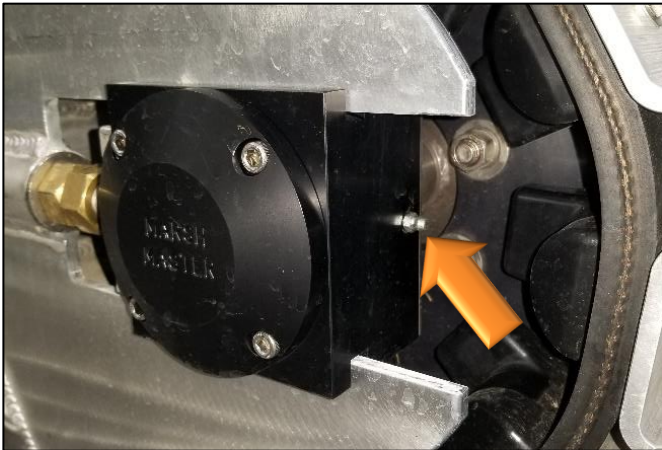
DAILY-7: Front Track Grease Port
