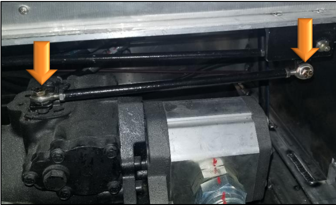
250 HOURS-4: Control Rods
