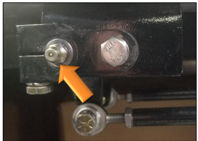
250 HOURS-3: Detent Shaft Grease Port
